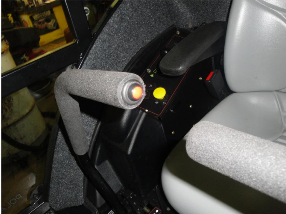
**Figure 2** – Push button harness installed and foam grip cut
