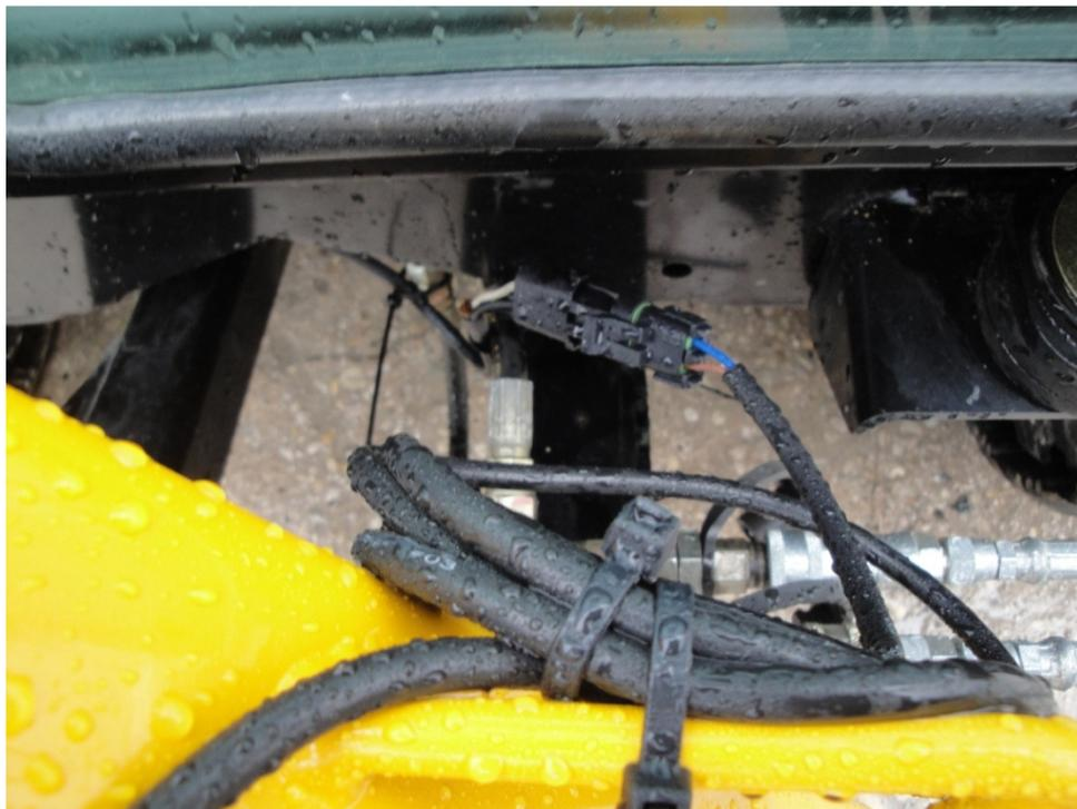
**Figure 3** – Adapter Harness Connected to Attachment Harness
