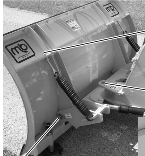
Loosen to Remove Spring
