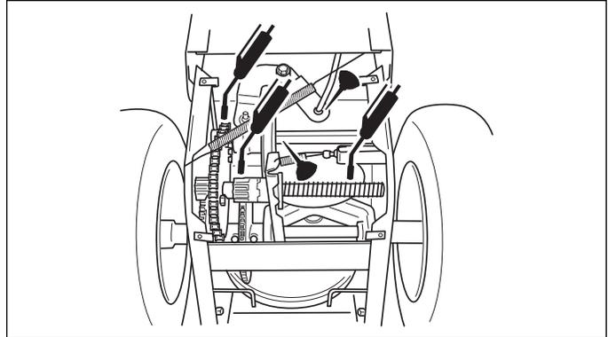
Figure 10. Drive Lubrication
