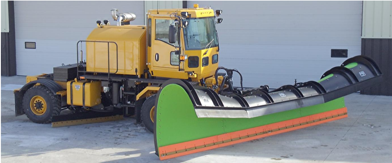
Shown with optional reversible plow, underbody scraper and fifth wheel hitch with steel ballast
