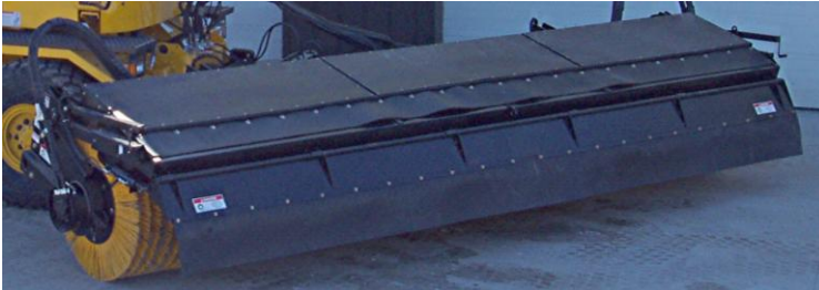
Shown on Front Mount Broom: No air blowers on broom head but with adjustable deflector
