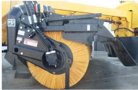
Shown on MB5 Mid-Mount Broom: Air blowers on broom head and non-adjustable deflector
