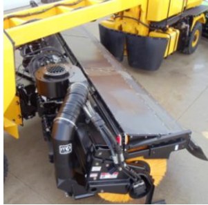
Shown on MB5 Mid-Mount Broom: Air blowers on broom head and non-adjustable deflector
