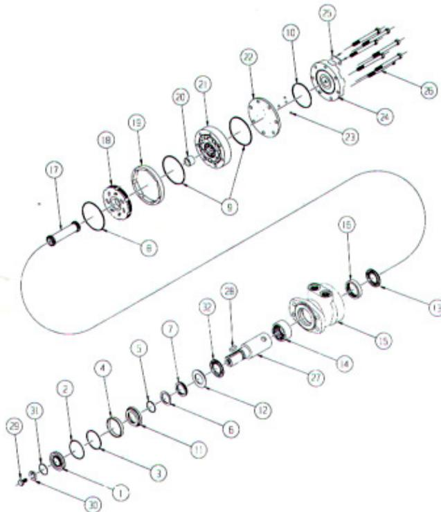
\*Note-Motor shaft shown with keyway, actual shaft has a spline.
