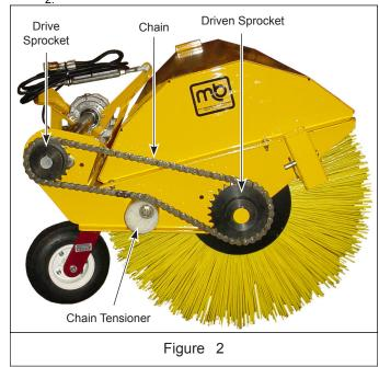
Remove chain half-link and clip to disconnect chain ends. Remove drive chain. See Figure 3.
