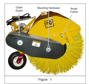
Loosen 1/2-13 x 3-3/4" socket head capscrew attaching chain tensioner and rotate tensioner until chain is slack. See Figure
