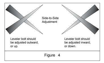
Broom head may be either pitched down too far forward or up too far backward on either side swing arm, giving us the impression of a bowtie. The swing frame bolts must be adjusted either out or in, either separately or together, to achieve a balanced pattern. See Figure 5.
