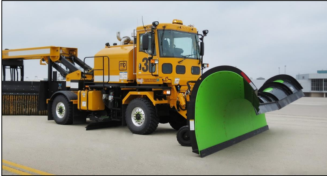
Reference Only: Shown with cradle, fifth wheel hitch, 24-foot reversible flared plow and underbody scraper
