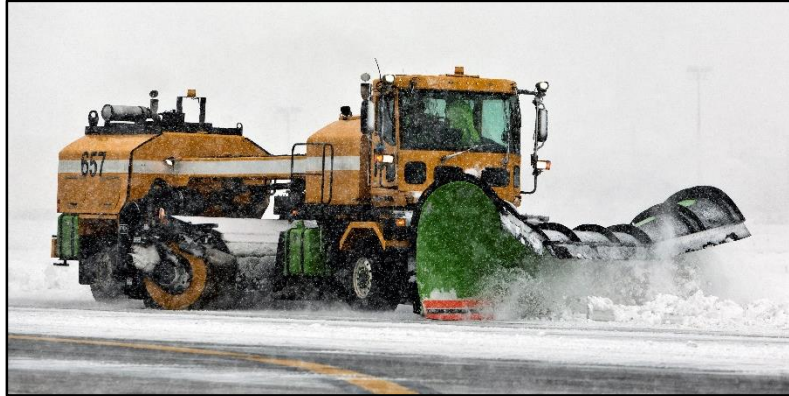
Reference Only. Shown with optional 24 Ft flared plow & 22 Ft broom
