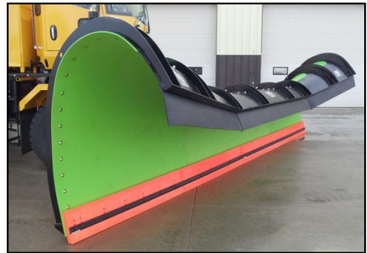
Plow with option flared end, optional poly edge
