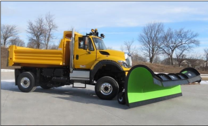
4 x 4 with Host Chassis and optional reversible plow and dump body
