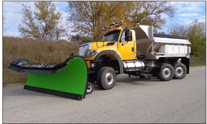
6 x 6 with Host Chassis and optional plow and pre-wet spreader body
